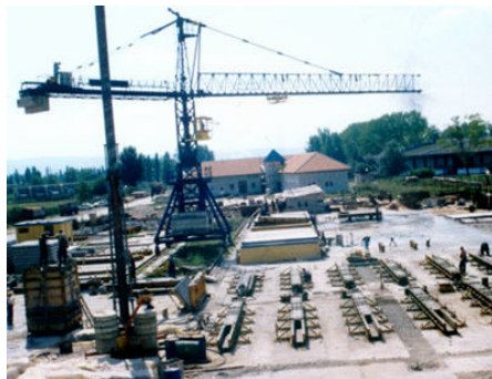
Polygon for element production – Novi Sad Concrete plant at the polygon – Novi Sad
